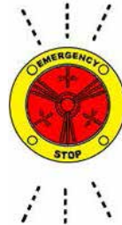
Pulsante + luce lamp. te lenta Button + slow flashing light
